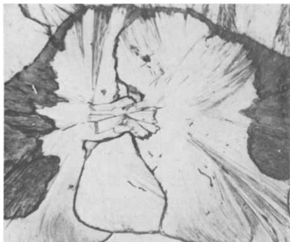
Figure 23 —A solid-solid polymorphic transformation taking place in a thin crystalline film of vanillin. The darker area (pseudomorph) is an area originally unstable and now converted to the stable form.
